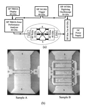
FIG. 1. (a) Schematic diagram of experimental setup for measuring the drain-source current transient characteristics of HFETs up to 40 GHz. The probing contact is shown inside the dotted ellipse. (b) Scanning electron microscopy images of HFET structures used in this work.
