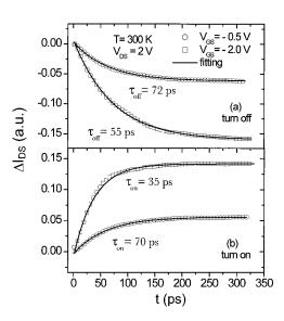
FIG. 3. Drain current transient kinetics of (a) switching-on and (b) switching-off at two representative gate-source voltages. Measured data points have been deconvoluted from the system response. Solid lines are the least squares fitting of data to the functions,  $\Delta I = \Delta I_0 [1 - \exp(-t/\tau_{on})]$  for the on process and  $\Delta I = \Delta I_0 [\exp(-t/\tau_{off}) - 1]$  for the off process.
