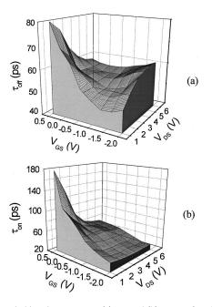
FIG. 4. The switching time constant. (a)  $\tau_{\rm off}$  and (b)  $\tau_{\rm on}$ , as functions of the to P gate-source bias  $V_{\rm GS}$  and drain-source bias  $V_{\rm DS}$ .
