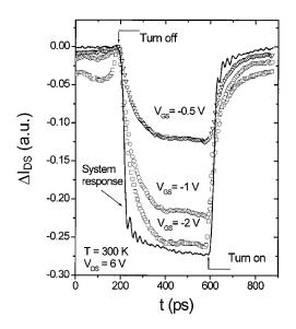
FIG. 2. Drain-source current transient behaviors (or switching-on and -off characteristics) of HFET A measured at T=300 K under a fixed dc drainsource bias ( $V_{DS}=6$  V) for three representative pulsed gate-source voltages  $V_{GS}$ . The system response to the input picosecond square wave pulse is also included and indicated as system response.
